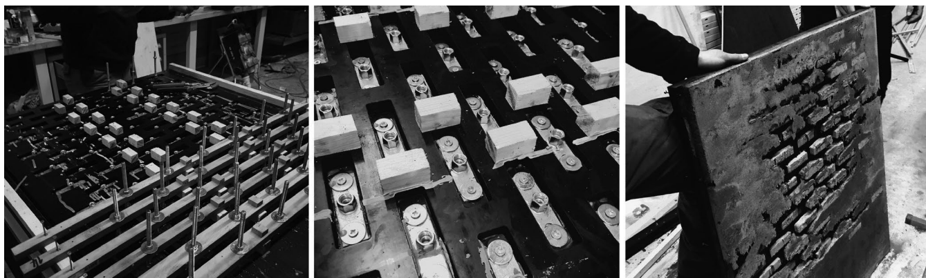
Figure 3: Punch Card method was not easy to demold, resulting in most of the wood staying in the cast. (Photographs by author.)
